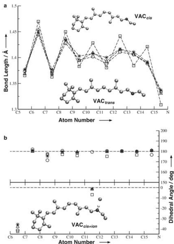
**Figure 2.** RPSB in vacuo: a) bond lengths and b) dihedral angles for optimized structures (atoms numbered according to Figure 1).  $VAC_{cis}$  (\*),  $VAC_{B3LYP}$  ( $\Delta$ ),  $VAC_{trans}$  (○),  $VAC_{cis+ion}$  (□).
